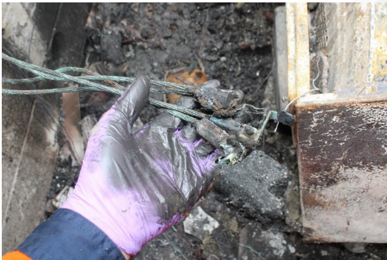
Photograph 14: The remains of the electricity meter, inside the sanitation unit.
