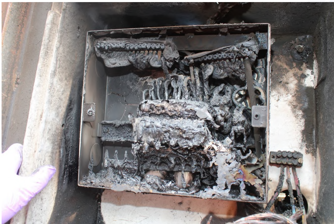
Photograph 16: A view of the remaining plastic inside the consumer unit.
